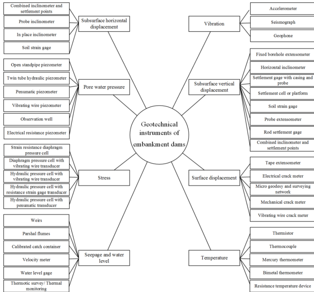
Fig. 5 Classified geotechnical instruments of embankment dams
