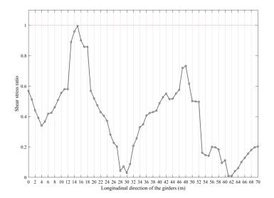
Fig. 8 Shear stress limitations of webs of each section for optimal design obtained by LPOA
