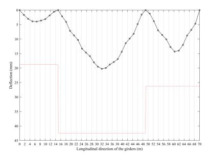
Fig. 10 Deflection limitations of the composite bridge for optimal design obtained by LPOA
