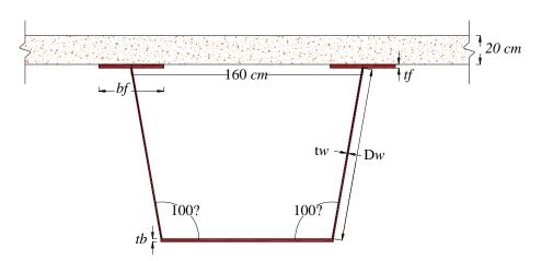
Fig. 4 A typical section of trapezoidal steel box girder
