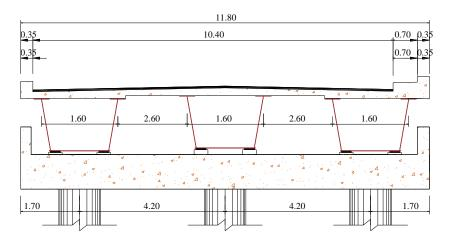
Fig. 2 A cross-sectional view of the composite steel box girder bridge
