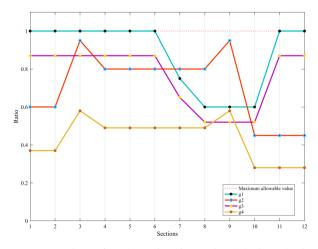
Fig. 6 Geometry constraints of each section for optimal design obtained by LPOA
