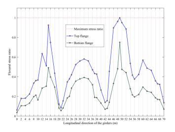
Fig, 7 Flexural stress constraints of the top and bottom flanges of each section for optimal design obtained by LPOA
