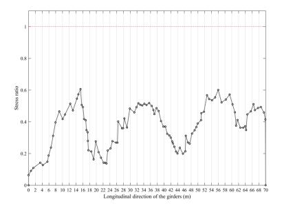
Fig. 9 Compressive stress limitations of the concrete slab for the optimal design by LPOA
