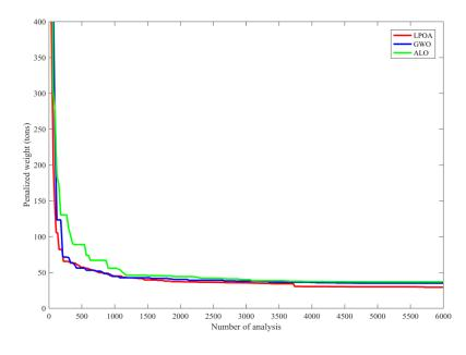
Fig. 5 Comparative of the convergence curves of LPOA, GWO, and ALO for the design of the multi-span composite box girder bridge
