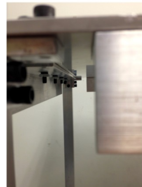
(b) Enlarged photo of the bolts and the nuts used to connect the stiffeners to the plates.
