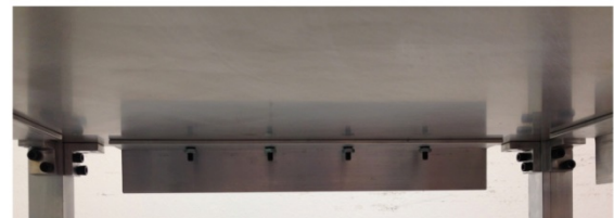
(a) A sample stiffener attached underneath one of the plates. The angle-brackets used to connect the columns to the plates can be seen on the sides.
