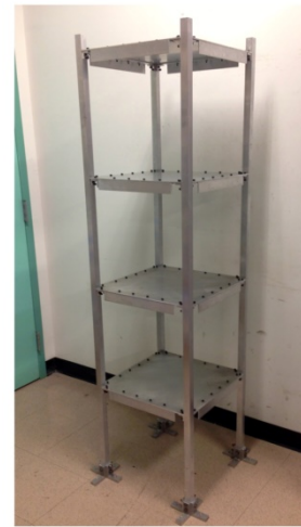
(a) A photo of the four-story experimental test-bed structure.
