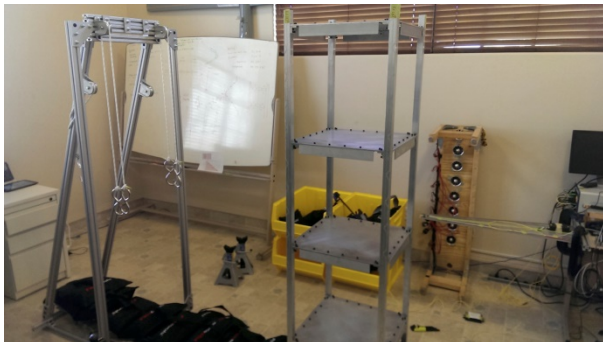
(b) Photo of the actual structure and the pulley system for load application.
