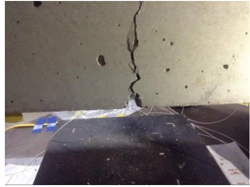
Fig. 19 Cracking process of concrete mold during the experiment
