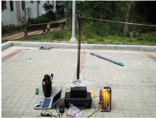
Fig. 11 Experiment setup for measuring ground temperature
