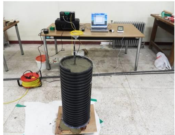
Fig. 5 Model rock body and monitoring devices
