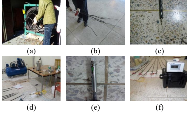
Fig. 14 Manufacturing process of FBG embedded tendon: (a) Cut the 7-wire strand, (b) Dismantle the strand and replace king cable, (c) Insert the optical fiber, (d) Insert the resin, (e) Protecting cap, (f) Test the FBG sensors
