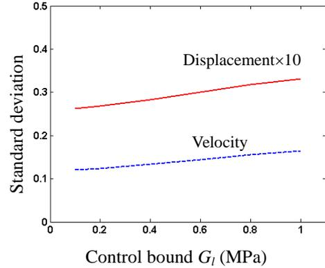
Fig. 14 Standard deviations of optimally controlled responses of MRVE sandwich beam under stochastic excitation versus control bound  $G_l$  ( $G_h=1.5$  MPa) (solid line: displacement  $\bar{w}$ ; dashed line: velocity  $\dot{\bar{w}}$ ).
