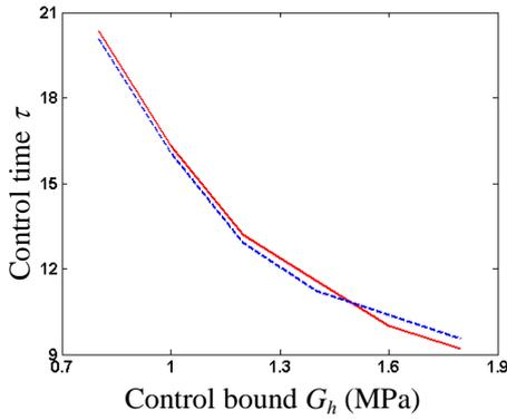
Fig. 5 Optimal control time  $\tau$  versus control bound  $G_h$  of MRVE sandwich beam under shock excitation (dashed line: controlled velocity response  $\dot{\bar{w}} < 0.0005$ ; solid line: controlled displacement response  $\bar{w} < 0.0001$ )
