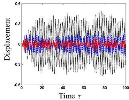
Fig. 8 Optimally controlled and passively controlled displacement responses of MRVE sandwich beam and displacement response of the beam without MRVE under stochastic excitation (dotted line: without MRVE; dashed line: passively controlled; solid line: optimally controlled)
