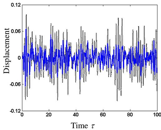
Fig. 10 Optimally controlled displacement responses of MRVE sandwich beam under stochastic excitation for different control bounds (dotted line:  $G_h=1.0$  MPa; solid line:  $G_h=3.0$  MPa)
