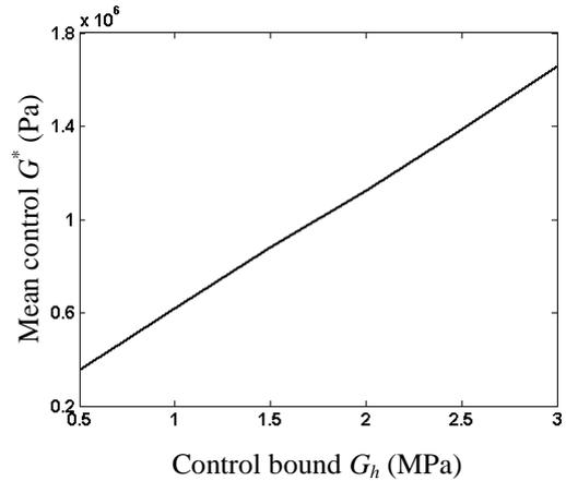
Fig. 13 Mean optimal control versus control bound  $G_h$  for stochastic excitation
