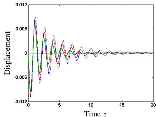
Fig. 4 Optimally controlled displacement responses of MRVE sandwich beam under shock excitation for different control bounds (dotted line:  $G_h=0.8$  MPa; dashed line:  $G_h=1.0$  MPa; solid line:  $G_h=1.4$  MPa)
