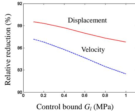
Fig. 15 Relative reductions in standard deviations of optimally controlled responses of MRVE sandwich beam under stochastic excitation versus control bound  $G_l$  ( $G_h=1.5$  MPa) (solid line: displacement  $\bar{w}$ ; dashed line: velocity  $\dot{\bar{w}}$ ).
