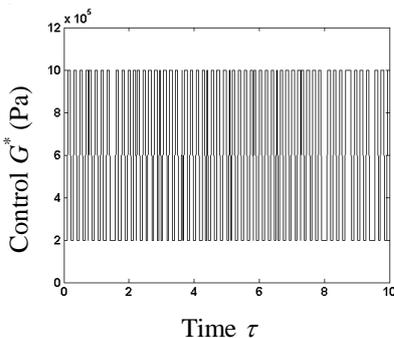
Fig. 3 Optimal bounded parametric control varying with time for shock excitation
