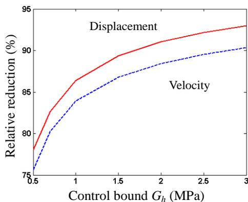
Fig. 12 Relative reductions in standard deviations of optimally controlled responses of MRVE sandwich beam under stochastic excitation versus control bound  $G_h$  ( $G_l=0.2$  MPa) (solid line: displacement  $\bar{w}$ ; dashed line: velocity  $\dot{\bar{w}}$ )
