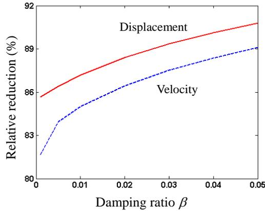
Fig. 17 Relative reductions in standard deviations of optimally controlled responses of MRVE sandwich beam under stochastic excitation versus damping ratio  $\beta$  (solid line: displacement  $\bar{w}$ ; dashed line: velocity  $\dot{\bar{w}}$ )
