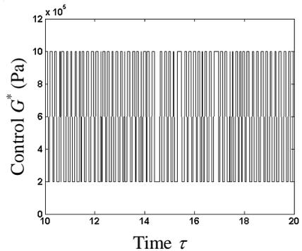
Fig. 9 Sample of optimal bounded parametric control varying with time for stochastic excitation
