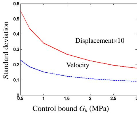
Fig. 11 Standard deviations of optimally controlled responses of MRVE sandwich beam under stochastic excitation versus control bound  $G_h$  ( $G_l=0.2$  MPa) (solid line: displacement  $\bar{w}$ ; dashed line: velocity  $\dot{\bar{w}}$ )
