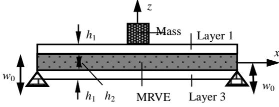
Fig. 1 Sandwich beam with MRVE core and supported mass
