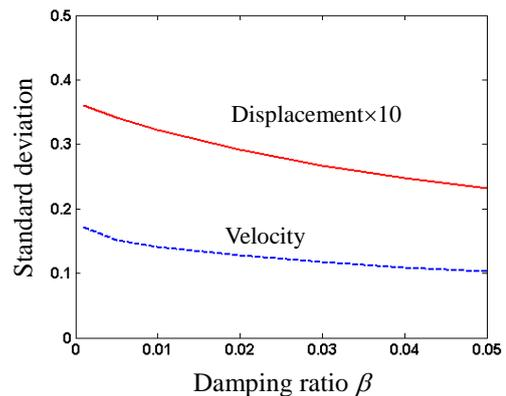
Fig. 16 Standard deviations of optimally controlled responses of MRVE sandwich beam under stochastic excitation versus damping ratio  $\beta$  (solid line: displacement  $\bar{w}$ ; dashed line: velocity  $\dot{\bar{w}}$ ).
