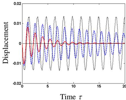
Fig. 2 Optimally controlled and passively controlled displacement responses of MRVE sandwich beam and displacement response of the beam without MRVE under shock excitation (dotted line: without MRVE; dashed line: passively controlled; solid line: optimally controlled)
