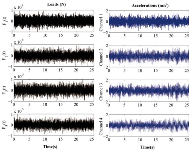
Fig. 3 Loads and measured accelerations in a certain test. Left column: applied ambient force on each floor slab; right column: measured acceleration signal of each accelerometer
