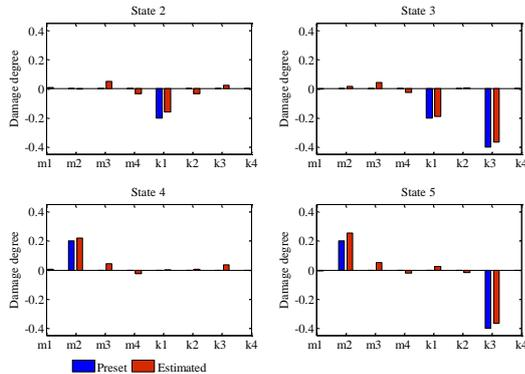
Fig. 6 Damage detection for four states under noisy environment (SNR = 5%)
