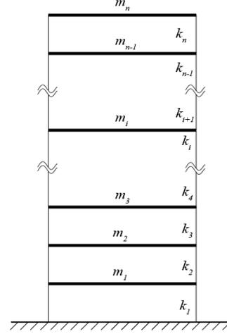
Fig. 1 Diagram of an  $n$ -story shear building
