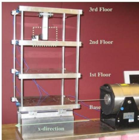
Fig. 9 LANL-4 DOF test-bed structure experiment
