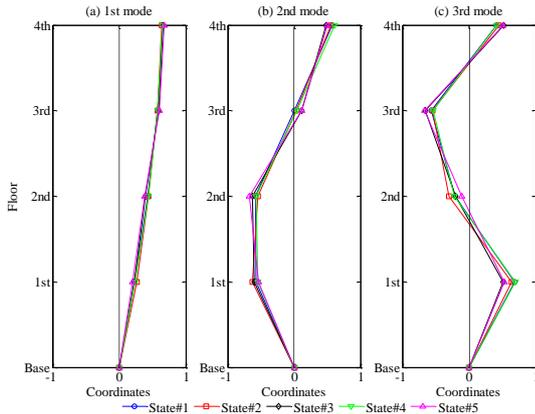
Fig. 4 Identified mode shapes for five test conditions of the numerical model
