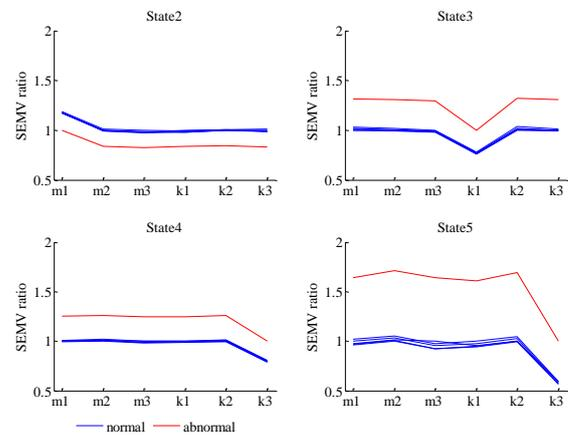
Fig. 11 SEMV solution matrix  $\mathbf{U}$  in four damage states
