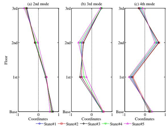
Fig. 10 Experimental mode shape for five test conditions
