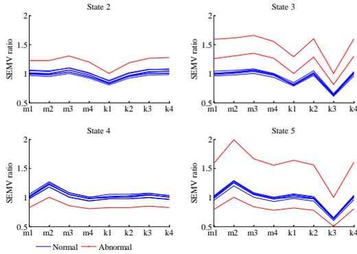
Fig. 5 SEMV solution matrix  $U$  for four damage states under noisy environment (SNR = 5%)
