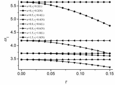
Fig. 8 The comparisons between fundamental frequencies of the simple supports by local model (L) and nonlocal model (N) with  $q=0$
