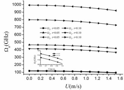
Fig. 9 Numerical example for the effect of axial velocity on circular natural frequencies including nonlocal and surface factors
