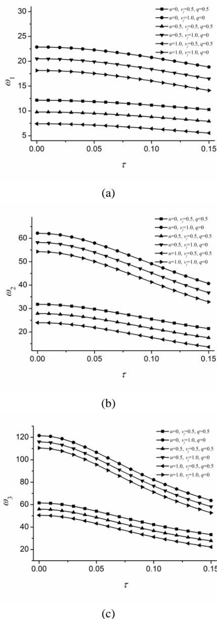
Fig. 3 Variations of the first three mode circular frequencies for the double-fixed supports
