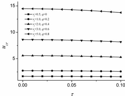
Fig. 7 Critical speed versus nonlocal nanoscale for simple supports
