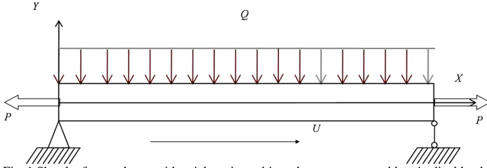
Fig. 1 Sketch of a nanobeam with axial motion subjected to transverse and longitudinal loads
