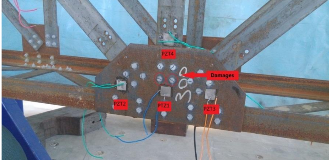
Fig. 4 The placed PZT sensors
