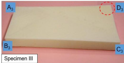
(c) Specimen III with upward distortion at corner D 3
