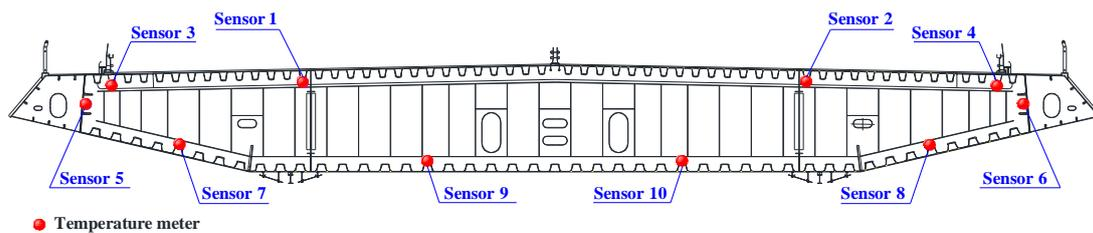
Fig. 13 Distribution of temperature meters on the middle section of the main span
