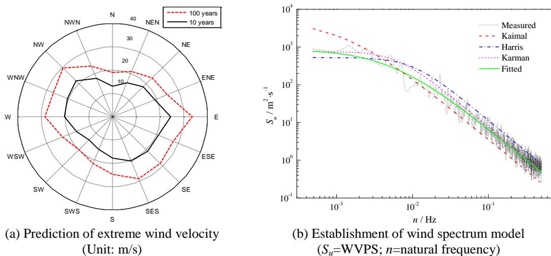
Fig. 11 Application of the monitored data in wind engineering
