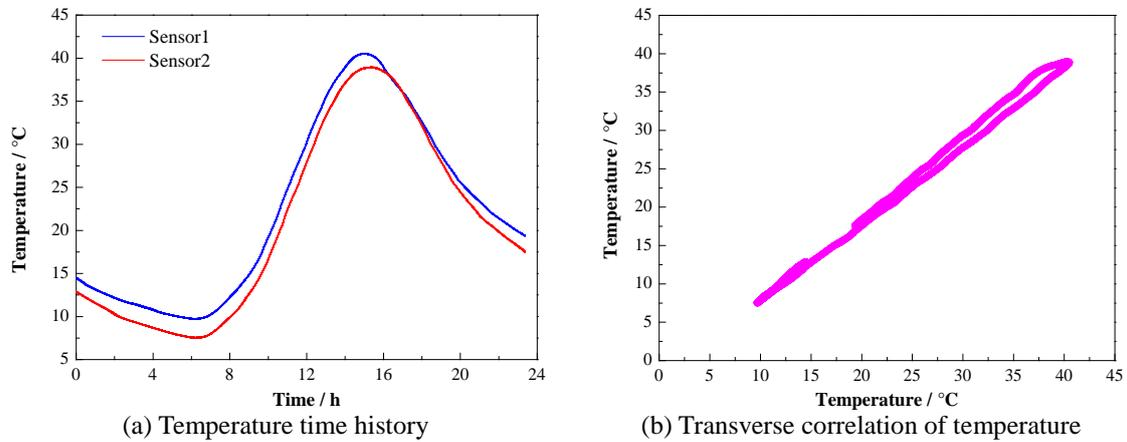
Fig. 12 Monitoring of the temperature on the steel box girder
