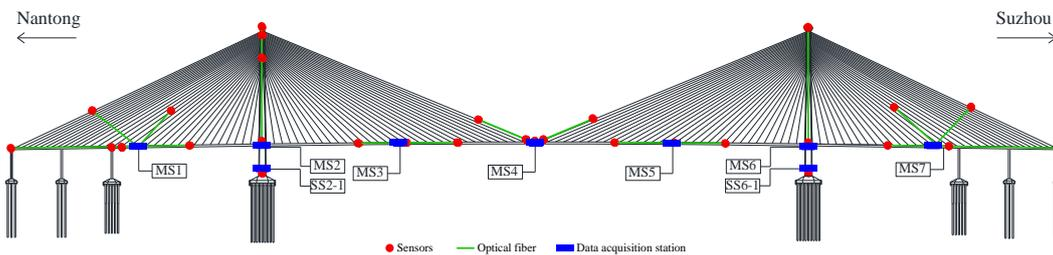
Fig. 7 Layout of the data acquisition station on SCB
