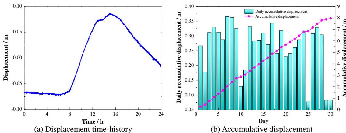
Fig. 16 Monitoring of the displacement for the expansion joint
