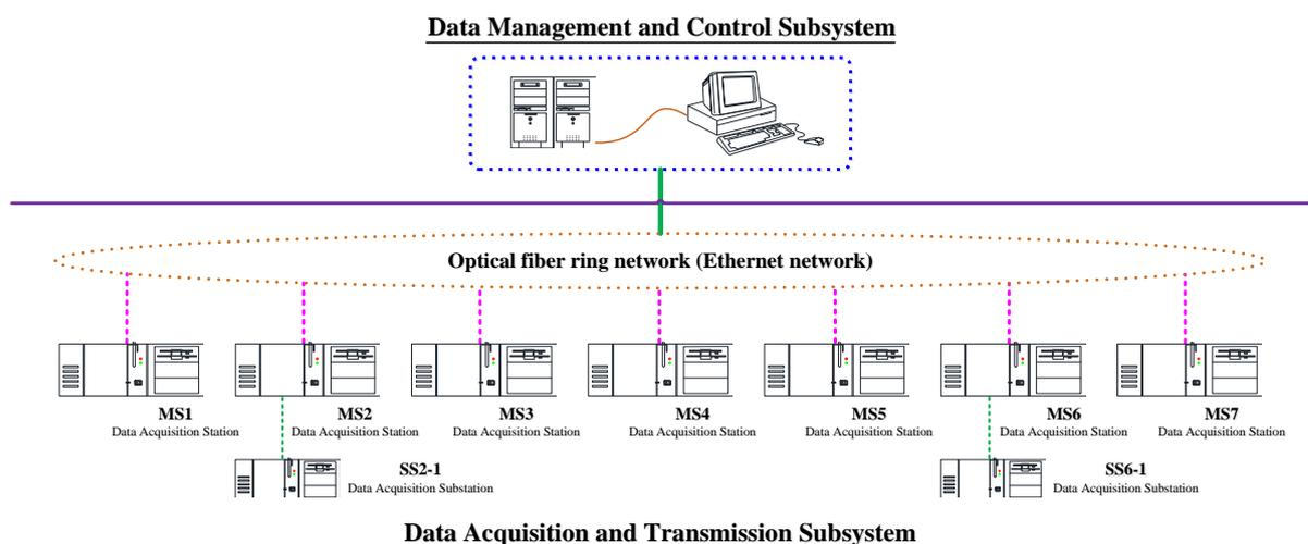
Fig. 6 Components of the Data Acquisition and Transmission Subsystem
