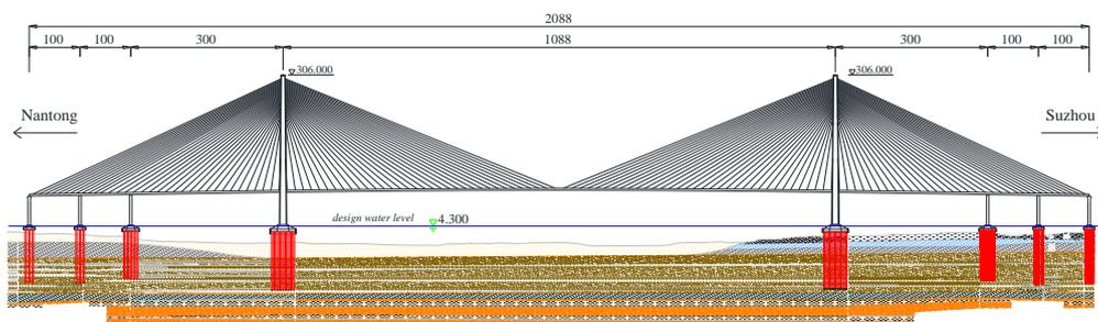
Fig. 1 Layout of the whole structure for SCB (Unit: m)
