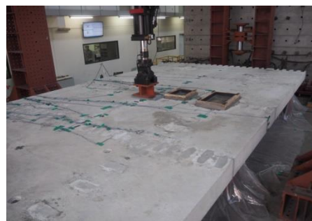
(h) Load application and leakage test
