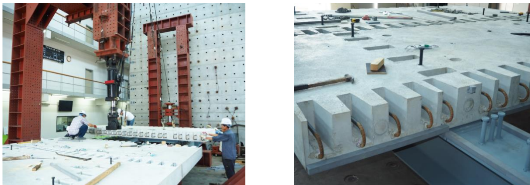
Fig. 2 Precast deck system with ribbed loop joints
