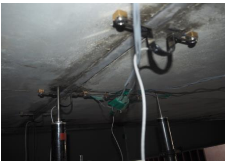
(g) Gauge installation at the bottom of deck
