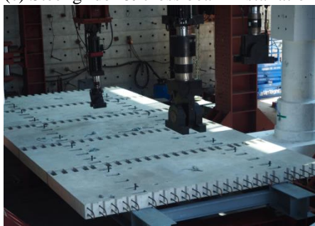
(e) Completion of PC deck installation
