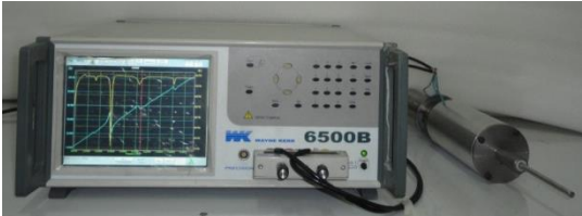
Fig. 9 Setup for impedance test
