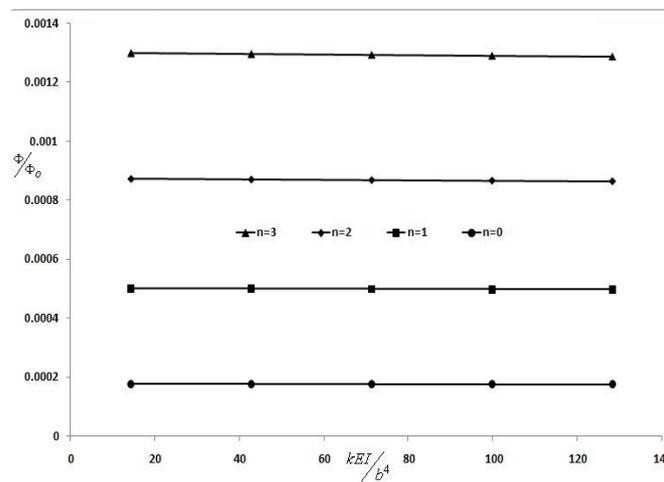
Fig. 4 The distribution of dimensionless electric potential in terms of dimensionless stiffness parameter for different non-homogenous indexes
