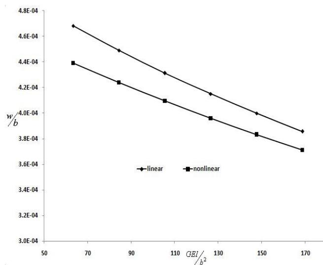
Fig. 7 Comparison between linear and nonlinear dimensionless transverse displacement in terms of dimensionless shear parameter
