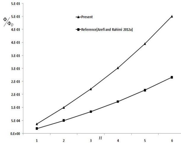
Fig. 12 The comparison between dimensionless electric potential of present and previous (Arefi and Rahimi 2012a) results
