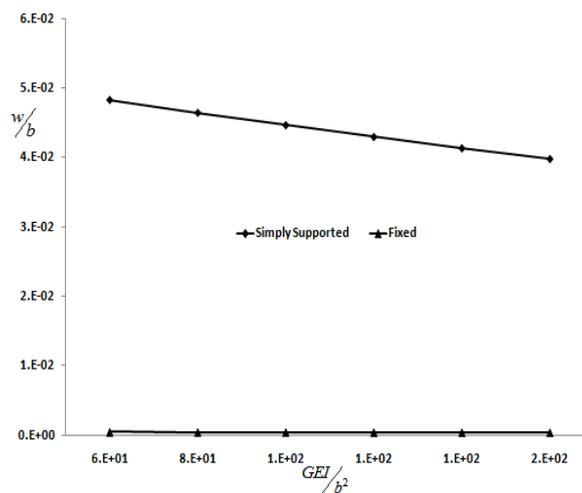
Fig. 10 The comparison between dimensionless transverse displacement of simply supported and fixed plate
