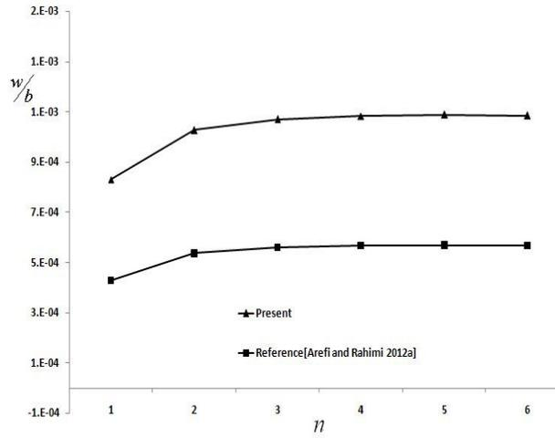
Fig. 11 The comparison between dimensionless transverse displacement of present and previous (Arefi and Rahimi 2012) a results
