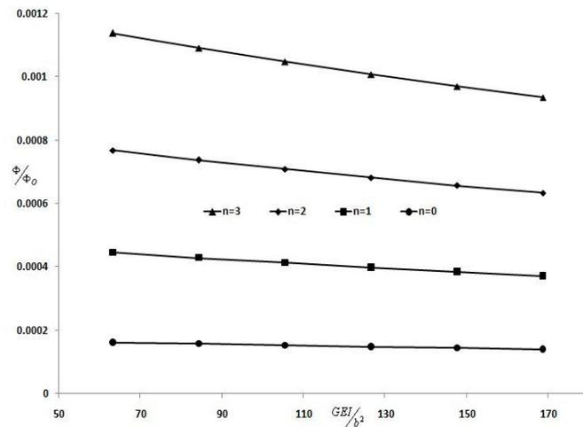
Fig. 5 The distribution of dimensionless electric potential in terms of dimensionless shear parameter for different non-homogenous indexes
