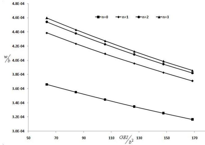
Fig. 3 The distribution of dimensionless transverse displacement in terms of dimensionless shear parameter for different non-homogenous indexes
