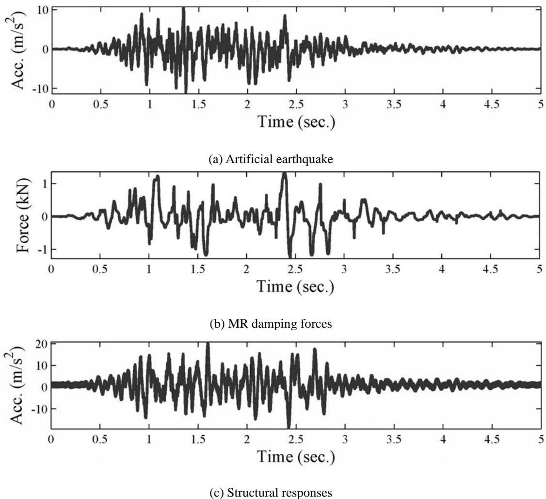
Fig. 6 A set of input and output for training the PANFIS model
