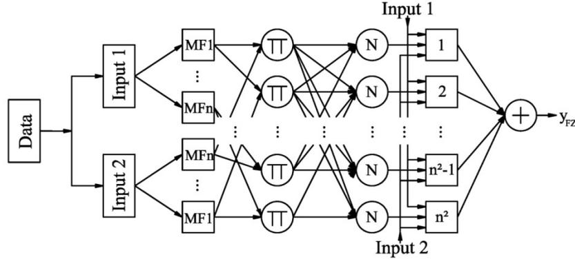
Fig. 2 ANFIS architecture with n MFs for each of the two inputs
