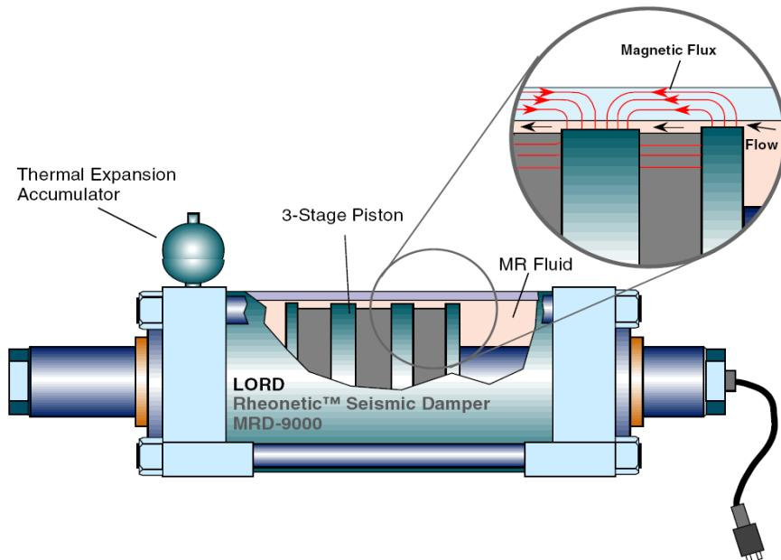
Fig. 5 Schematic of the prototype 20-ton large-scale MR damper (Yang *et al.* 2002)
