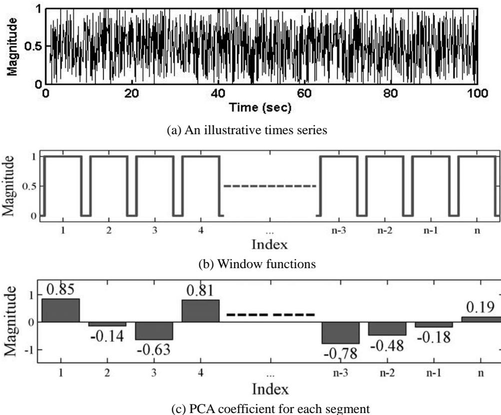
Fig. 3 Conceptual example on the application of PCA to times series
