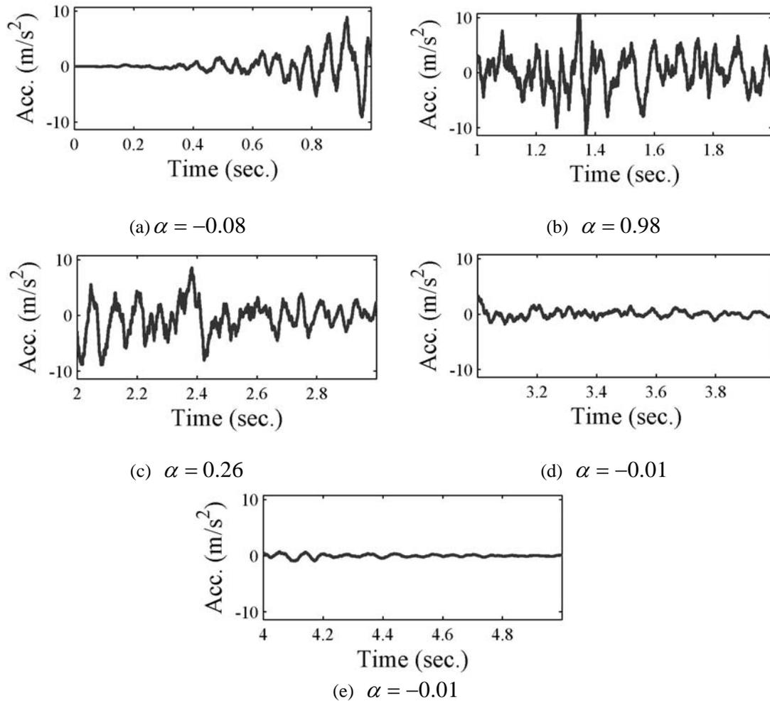
Fig. 7 Five segments of the artificial earthquake with corresponding PCA coefficients
