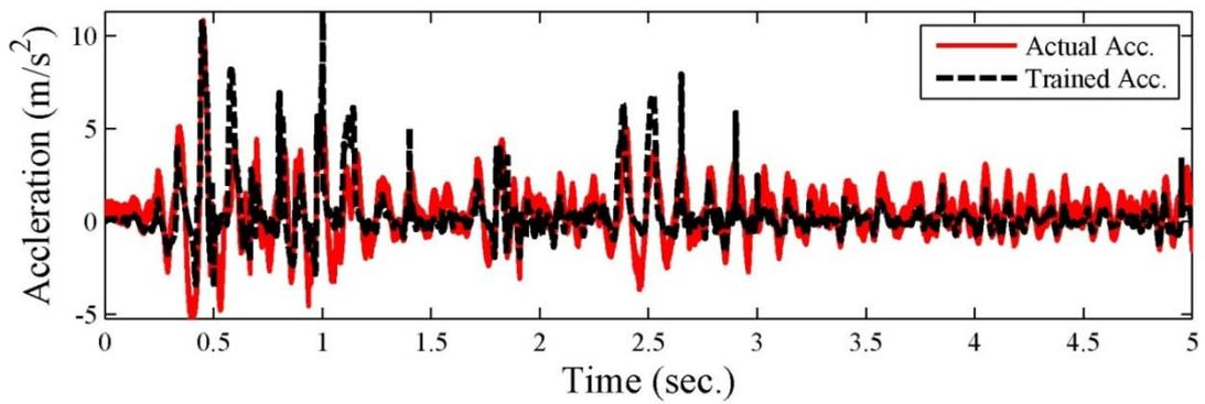
Fig. 9 Validation: El-Centro earthquake
