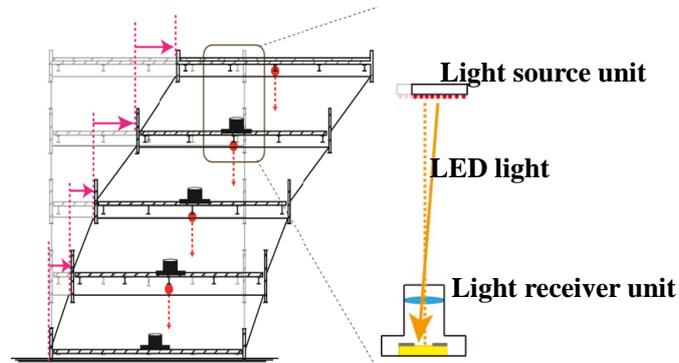
Fig. 1 Schematic illustration of drift displacement sensor
