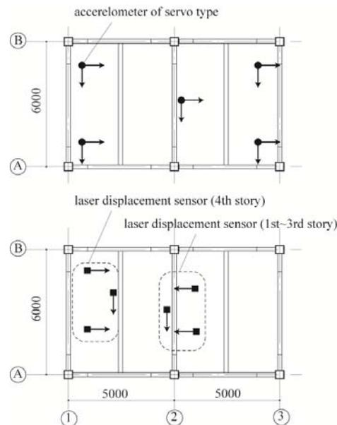
Fig. 4 Plan of model building with sensor locations
