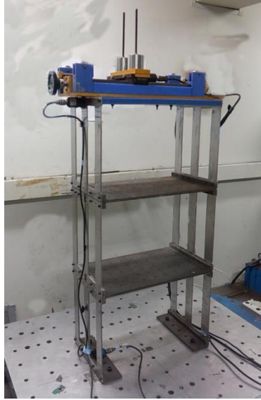
Fig. 3 Scaled 3-story shear building model
