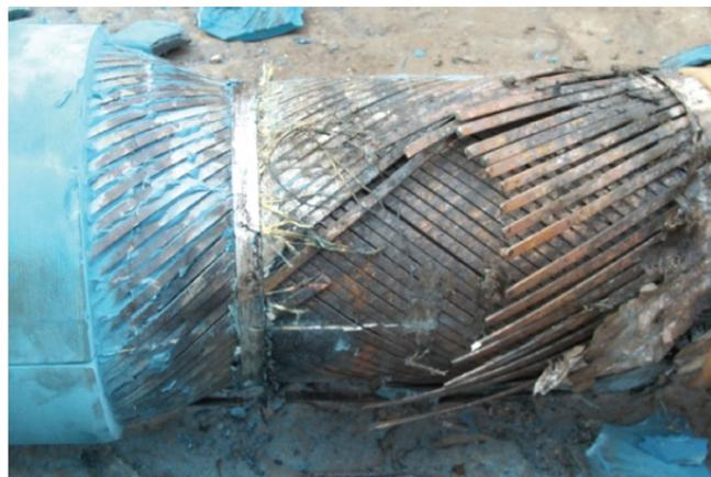
Fig. 1 End-fitting failure example (Pipa *et al.* 2010)
