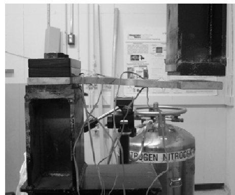
(b) Residual deformation of Plate-3, after the test
