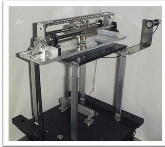
Fig. 6 Experimental test apparatus to implement semi-active impact damper approach
