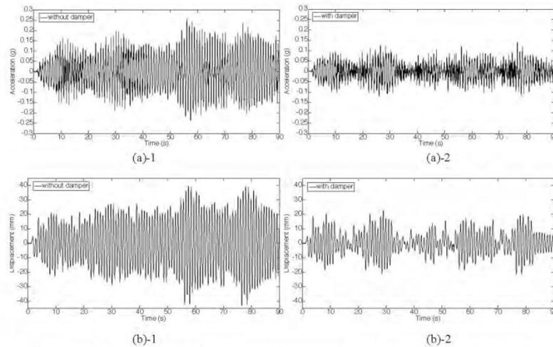
Fig. 5 Time-history plots of displacement and acceleration. (a)-1 and (b)-1: without control; (a)-2 and (b)-2: with particle dampers at the second and first floor, respectively, (Lu 2012)
