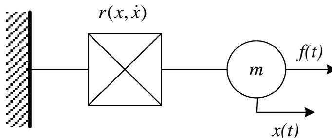
Fig. 1 Single degree of freedom system with nonlinear restoring force
