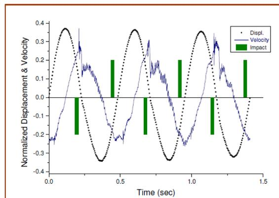
Fig. 7 Normalized displacement, velocity, and activation time of an experimental semi-active control device
