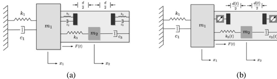
Fig. 2 Schematic representation of a highly-nonlinear auxiliary mass damper coupled to the primary system: (a) purely passive version; and (b) semi-active model
