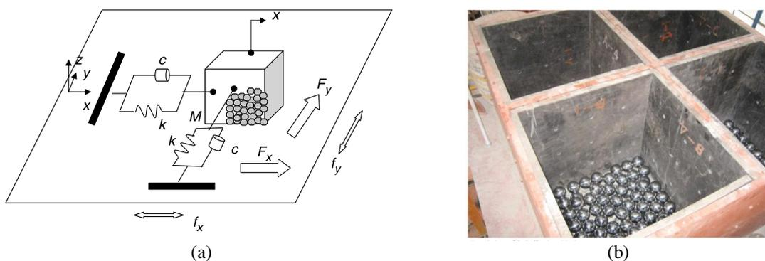
Fig. 4 Model of a particle damper: (a) schematic representation and (b) physical model used in (Lu 2012)
