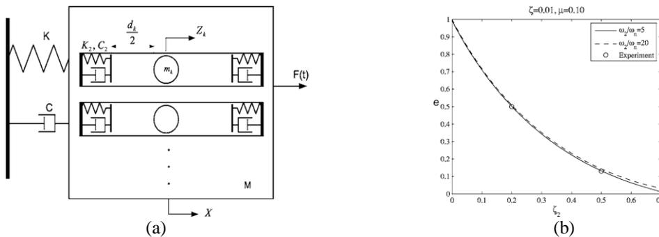
Fig. 3 The multiple-units impact damper: (a) schematic representation; and (b) dependence of the coefficient of restitution,  $e$ , on the damping parameter  $\zeta_2$  (Nayeri *et al.* 2007)
