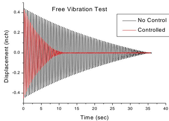
Fig. 8 Sample experimental results from a semi-active impact damper attached to a single-degree-of-freedom mechanical model
