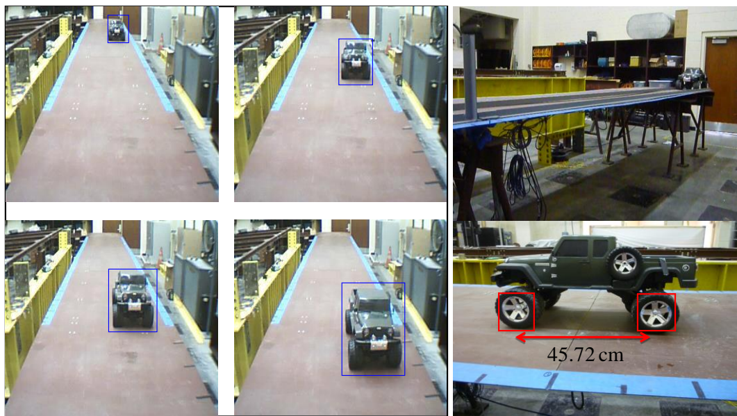
Fig. 7 Experimental test conducted on the 4-span bridge using radio controlled vehicle
