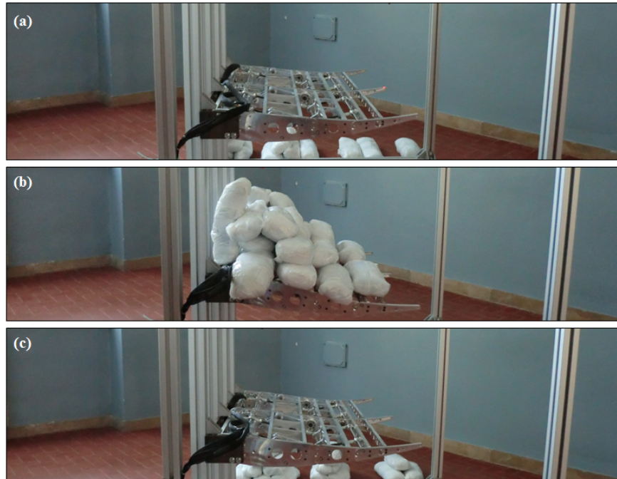
Fig. 17 Static test: (a) no load applied, (b) loaded structure and (c) un-loaded structure
