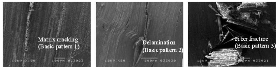
Fig. 13 Three basic damage patterns of BFRP specimens
