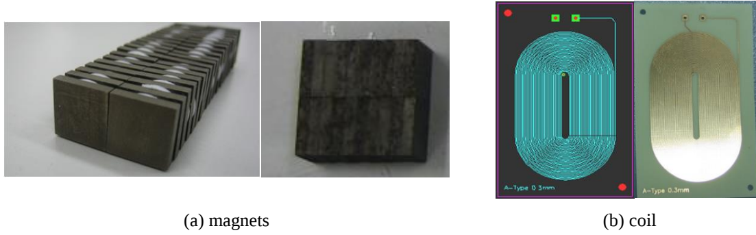
Fig. 10 Magnets and coil to construct EMAT
