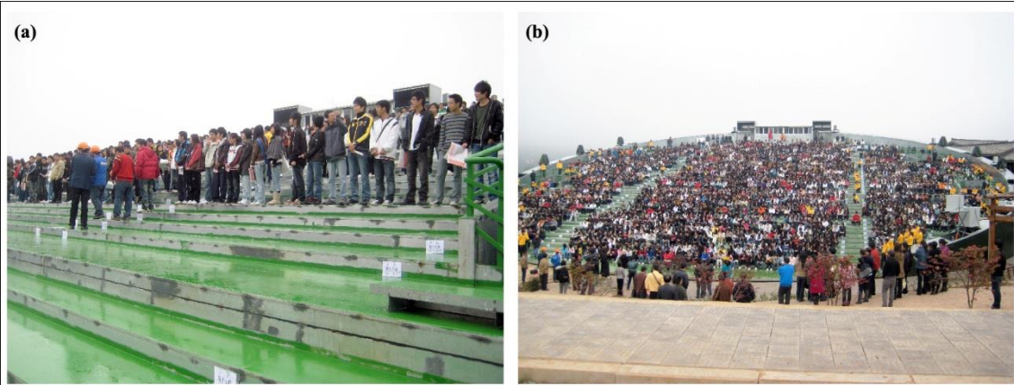
Fig. 18 Photos of test run carrying people: (a) 1000 people standing on the back-half region and the auditorium being ready to start; (b) Revolving with full load of 2000 people
