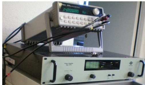
(c) Wave generator (top) and power amplifier (bottom)
