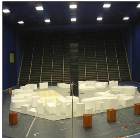
Fig. 8 A photograph of the wind tunnel test set up of the building and its surrounding (see Zasso *et al.* 2008 and Aly 2009)
