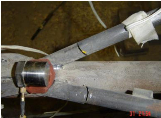
Fig. 11 100% damage of four web members
