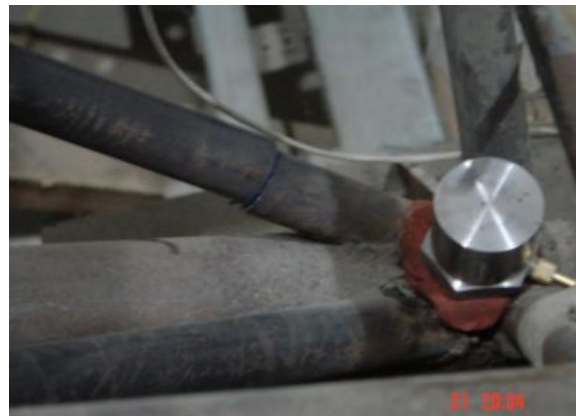
Fig. 10 100% damage of one end of web member 1
