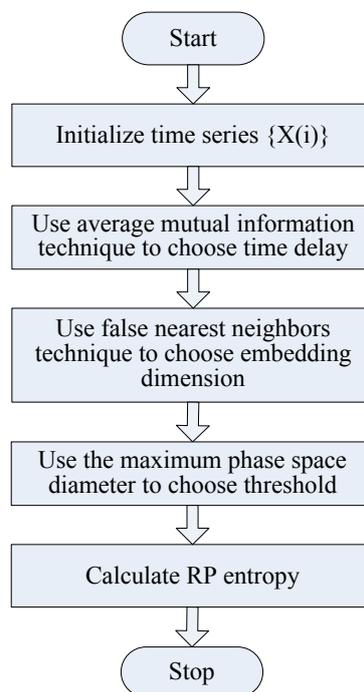
Fig. 5 Flow chart of recurrence plot entropy calculation
