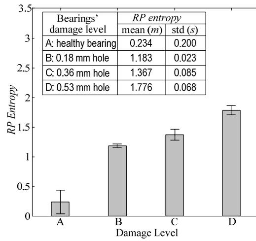
Fig. 9 RP entropy of vibration signals from four test bearings (Speed: 1,750 rpm; Load: 2HP)
