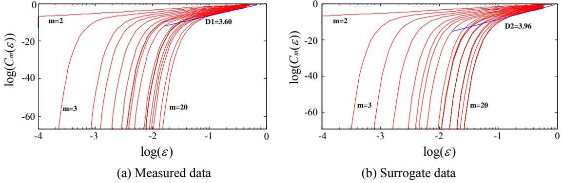
Fig. 3 Scaling behavior of measured data and surrogate data ( $m=2-20$  and  $\tau=2$ )
