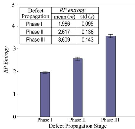
Fig. 11 RP entropy of vibration signals at different run-to-failure test stages
