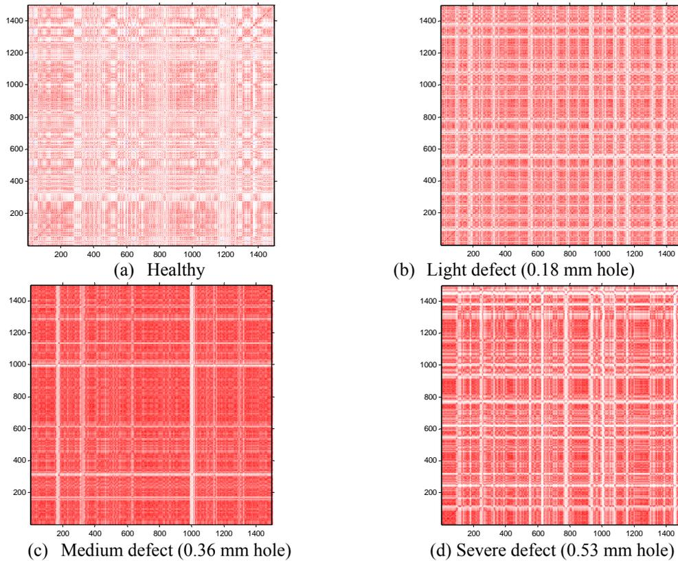
Fig. 7 Recurrence plots of vibration signals from four test bearings
