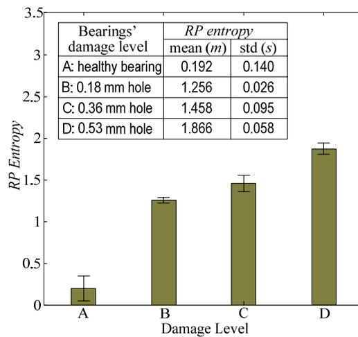
Fig. 8 RP entropy of vibration signals from four test bearings (Speed: 1,772 rpm, Load: 1 HP)
