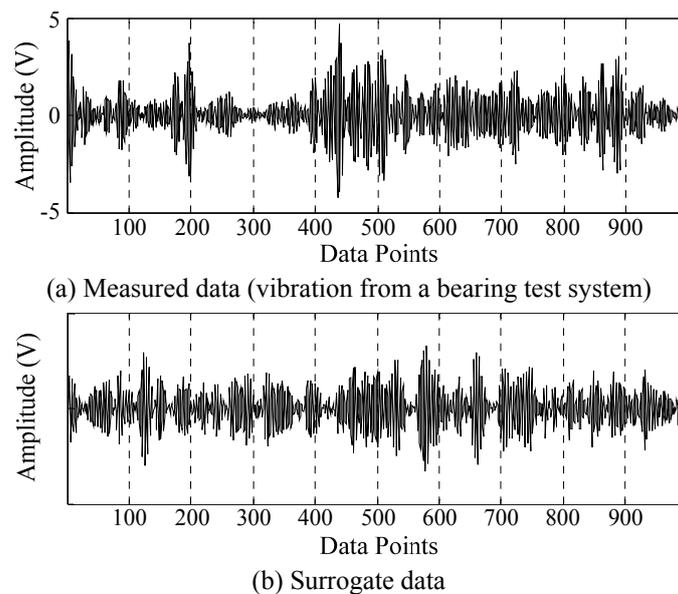
Fig. 2 Measured data and exemplary surrogate data used in non-linearity test
