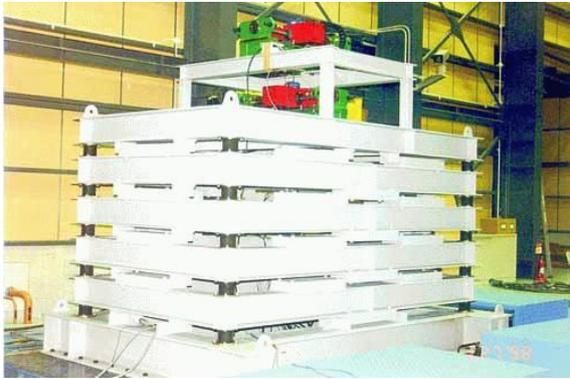
Fig. 7(a) A five layered structural model on a shaking table. Each mass of layer is supported by four base isolators at the four corners of each layer
