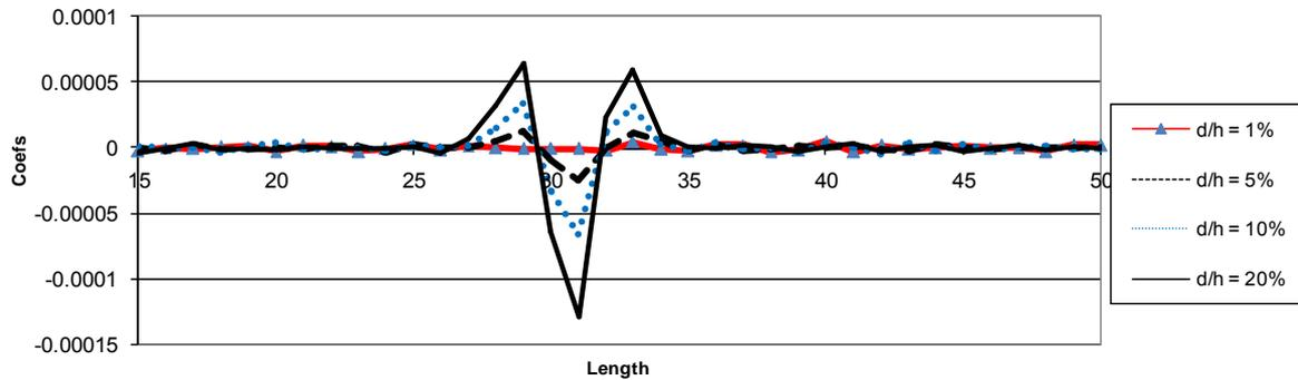
Fig. 10 Graph of WT coefficients for  $a = 2$  (Sym 4), with different ratios of  $d/h$
