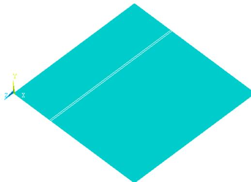
Fig. 7 Plate with size of  $1000 \times 1000 \times 10$  mm with crack at  $x_d = 300$  mm
