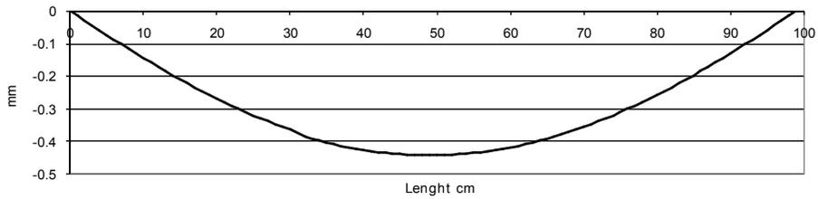
Fig. 4 Numerical representations of segmental displacement response with unequal interval of sampling points for undamaged plate along with plotted curve by 2D array
