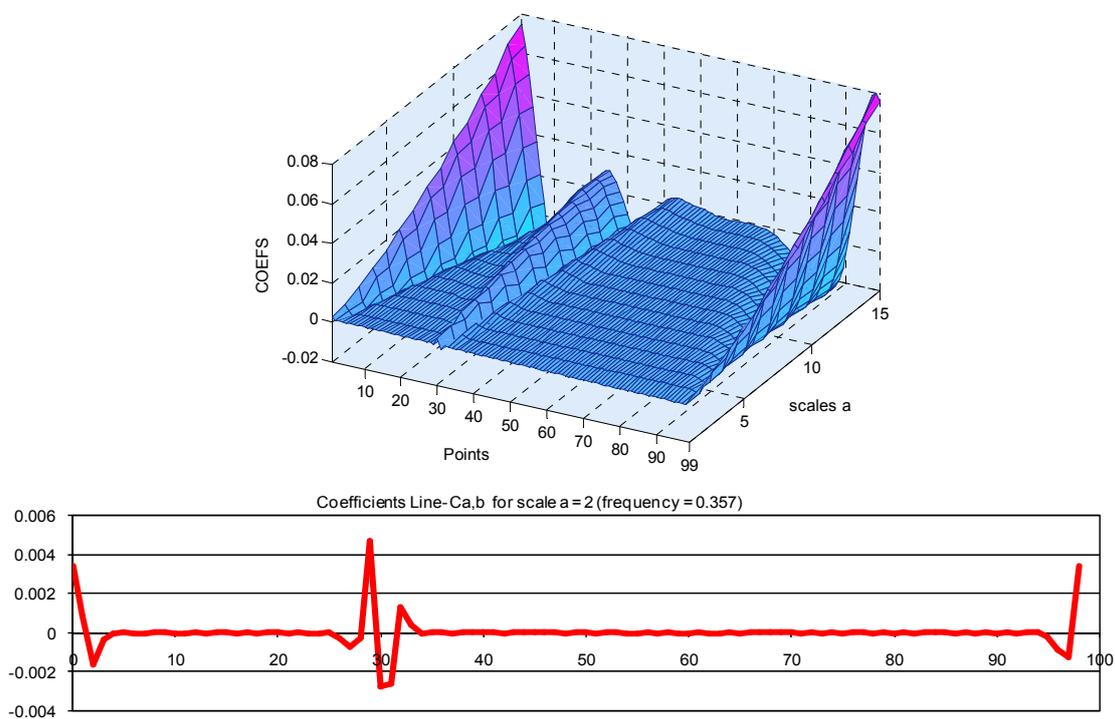
Fig. 6 3D and 2D Graph of WT coefficients of undamaged plate with Sym 4
