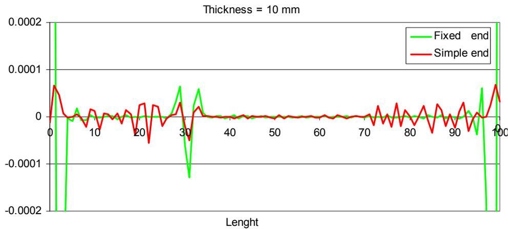
Fig. 15 Graph of WT coefficients ( $a = 2 / \text{Sym } 4$ ) for plate ( $h = 10 \text{ mm}$ ) with different boundary condition
