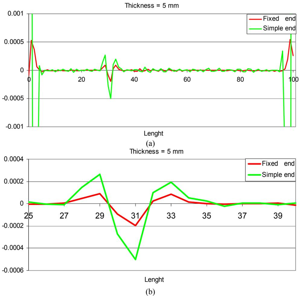
Fig. 14 (a) Graph of WT coefficients ( $a = 2$  / Sym 4) for plate ( $h = 5 \text{ mm}$ ) with different boundary conditions and (b) Close-up view of WT coefficients at damage locations
