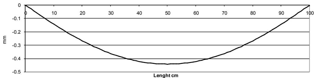
Fig. 2 Numerical representations of segmental displacement response with equal interval of sampling points for undamaged plate along with static response curve
