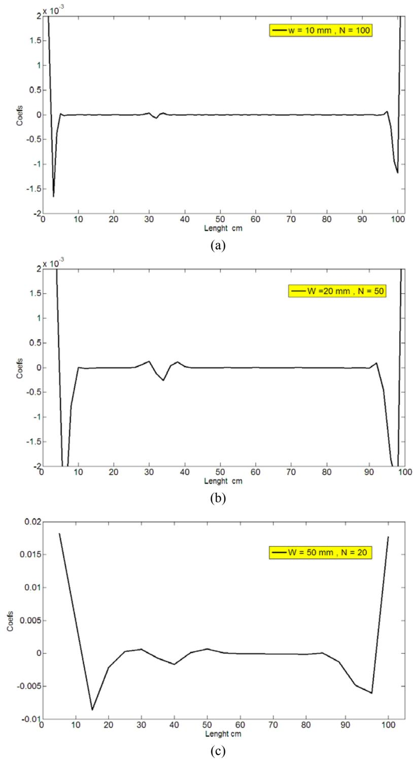
Fig. 11 Graph of WT coefficients for  $a = 2$  (Sym 4), with different cracks widths and different number of sampling points
