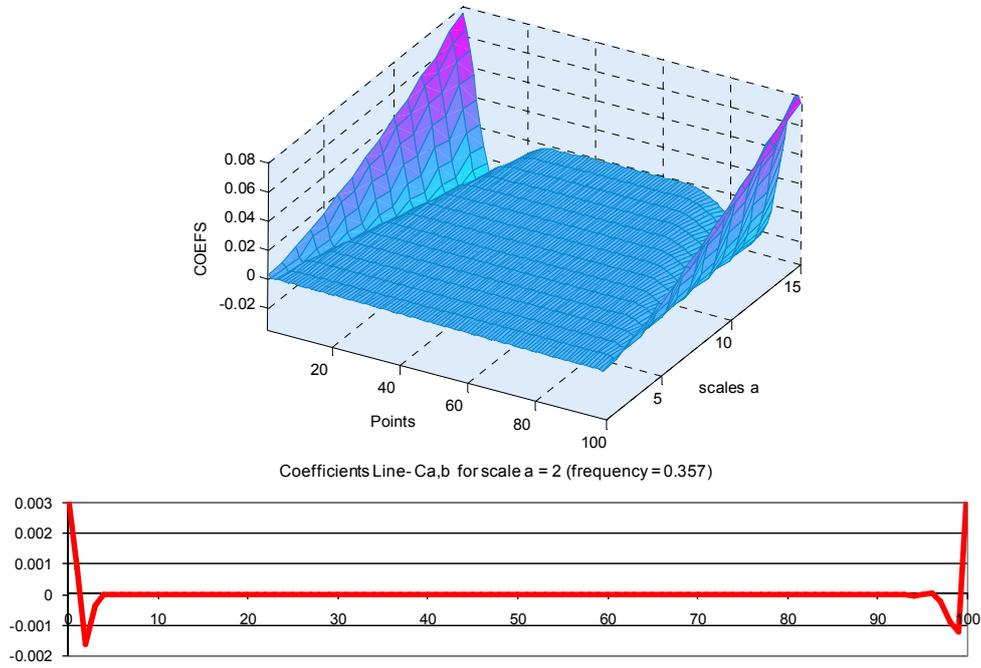
Fig. 3 3D and 2D graph of WT coefficients of response for undamaged plate with Sym 4
