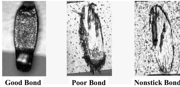
(b) The corresponding optical micrographs
