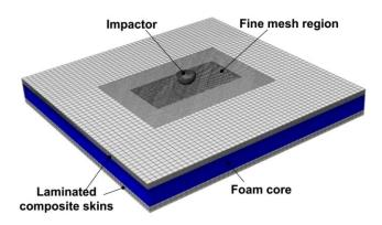
Fig. 3 FE model of sandwich panels
