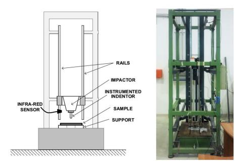
Fig. 1 Drop-weight testing machine used for impact testing
