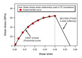
Fig. 2 Nonlinear shear stress-strain response of unidirectional layers implemented in the FE model
