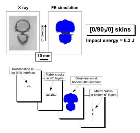
Fig. 11 Comparison of projected damage and through-thickness distribution of individual damage modes as obtained by X-ray and predicted by the FE model for a sandwich panel with  $[0/90_3/0]$  skins. Impact energy  $\approx 6.3$  J
