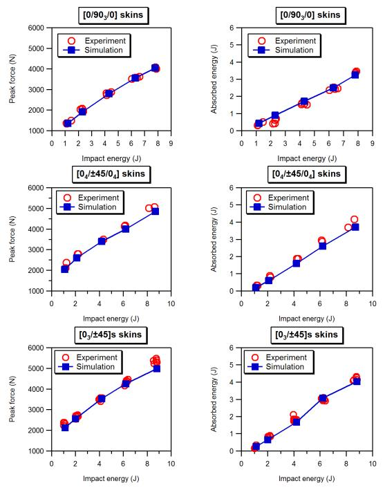
Fig. 9 Comparison between experimental and predicted peak contact forces (left column) and absorbed energies (right column) for sandwich panels with  $[0/90_3/0]$ ,  $[0_4/\pm 45/0_4]$  and  $[0_3/\pm 45]$ s skins
