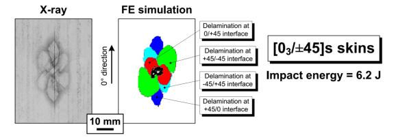
Fig. 13 Comparison of projected damage as obtained by X-ray and predicted by the FE model for a sandwich panel with  $[0_3/\pm 45]$ s skins. Impact energy  $\approx 6.2$  J. Different colours of the FE simulation correspond to different damage depths
