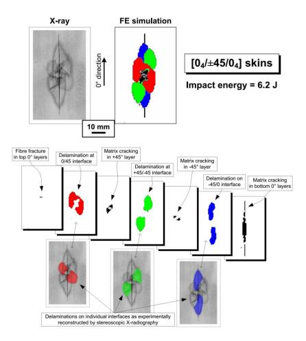
Fig. 12 Comparison of projected damage and through-thickness distribution of individual damage modes as obtained by X-ray and predicted by the FE model for a sandwich panel with  $[0_4/\pm 45/0_4]$  skins. Impact energy  $\approx 6.2$  J
