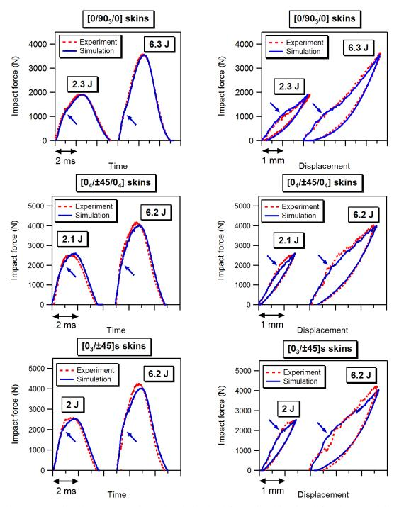
Fig. 8 Comparison between experimental and simulated force–time histories (left column) and force–displacement curves (right column) for sandwich panels with  $[0/90_3/0]$ ,  $[0_4/\pm 45/0_4]$  and  $[0_3/\pm 45]$ s skins impacted at two energy levels
