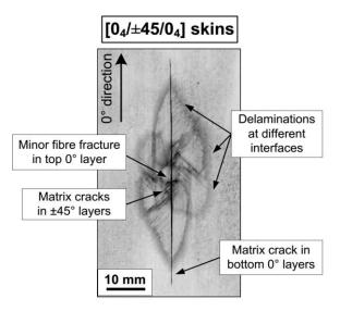
Fig. 6 X-ray of typical skin damage for sandwich panels with  $[0_4/\pm 45/0_4]$  skins. Impact energy  $\approx 6.2$  J
