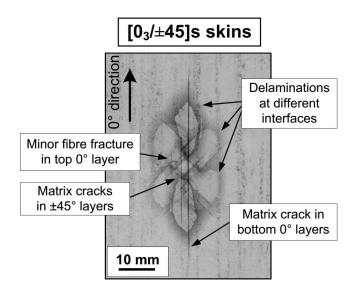
Fig. 7 X-ray of typical skin damage for a sandwich panels with  $[0_3/\pm 45]$ s skins. Impact energy  $\approx 6.2$  J
