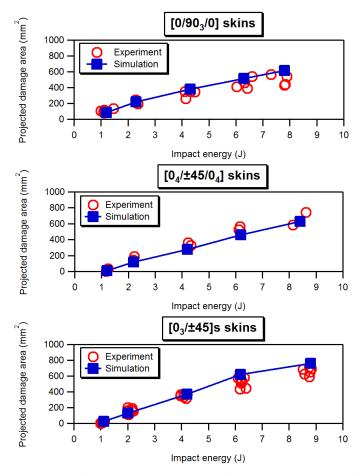
Fig. 10 Comparison between projected damage areas as obtained by X-ray and predicted by the FE model for sandwich panels with  $[0/90_3/0]$ ,  $[0_4/\pm 45/0_4]$  and  $[0_3/\pm 45]$ s skins impacted at various energies
