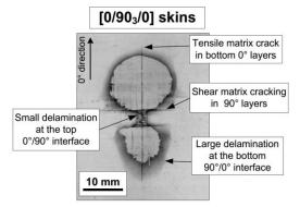
Fig. 5 X-ray of typical skin damage for sandwich panels with  $[0/90_3/0]$  skins. Impact energy  $\approx 6.3$  J
