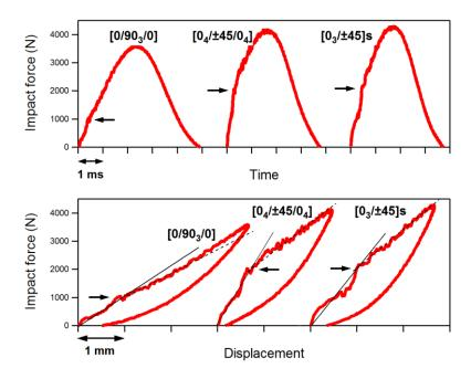
Fig. 4 Force-time and force-displacement curves of sandwich panels with  $[0/90_3/0]$ ,  $[0_4/\pm 45/0_4]$  and  $[0_3/\pm 45]$ s skins. Impact energy  $\approx 6.2$  J
