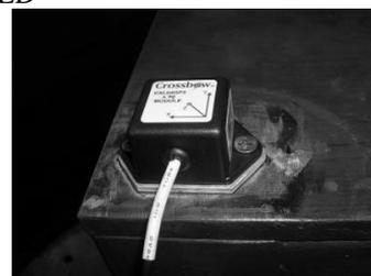
(c) wireless three dimensional acceleration transducer
