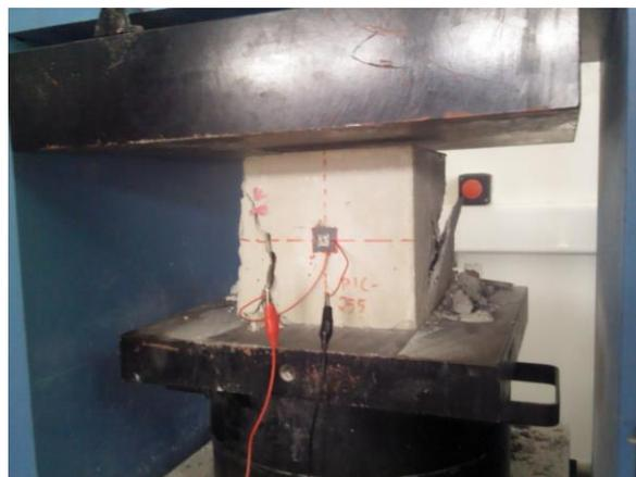
Fig. 6 Concrete specimen C2 on the compression machine (Failure)
