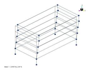
Fig. 9 Mode shapes  $1 - f_I = 2.88$  Hz
