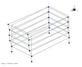
Fig. 10 Mode shapes  $2 - f_2 = 3.48$  Hz
