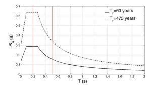
Fig. 12 Seismic input for Italian Technical Code: pseudo acceleration response spectra for soil category "C" at  $T_r = 50$  years and  $T_r = 475$  years - Vertical red lines defines the range in which fall the building natural periods
