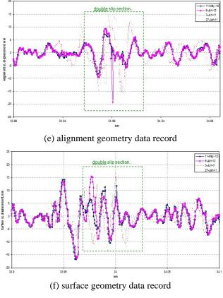
Fig. 12 AK Car geometry data
