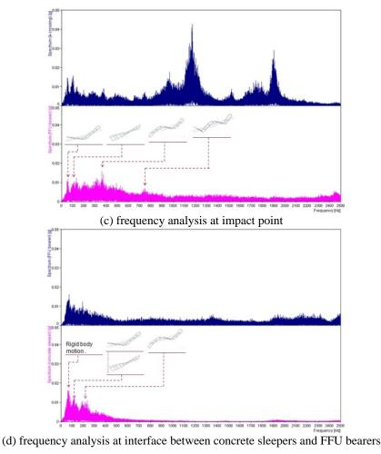
Fig. 14 Vibration data of a pass-by train (Passenger train, X-Up Main)
