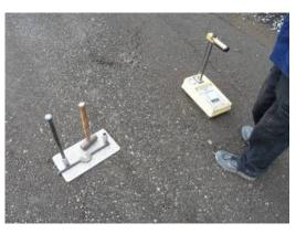
Fig. 8 Compaction test of capping layer
