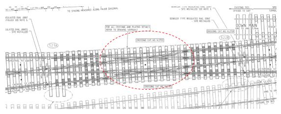
Fig. 4 Field layout of double slips (521/522) at Hornsby NSW
