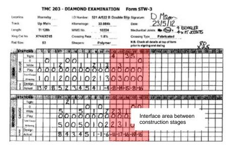
Fig. 11 Example of field inspection sheet of the double slips – showing good geometrical condition of turnout systems at the critical location
