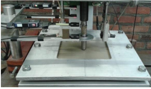
Fig. 2 Low velocity impact test on sandwich plate
