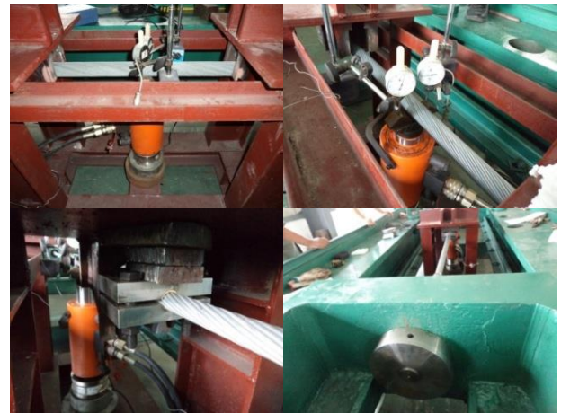
Fig. 8 Experiment of cable force identification
