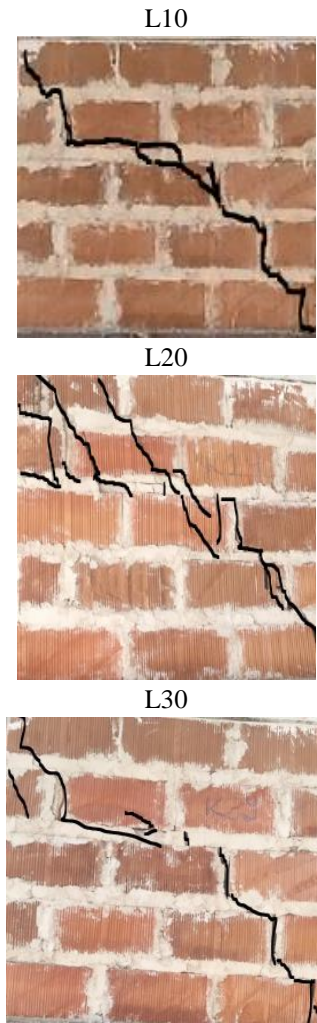
Fig. 5 Damages of the lime mortar walls
