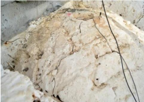
(b) Longitudinal crack on the top of the rib cover after loading.
