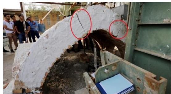
(a) Place of cracks in the vault, unreinforced structure
