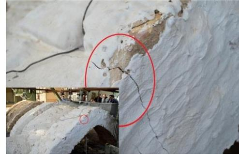
(a) Cracks in the vault under the load of 152 kN
