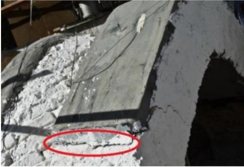
Fig. 16 Cracks at the junction of FRP to vaults under the load of 251 kN
