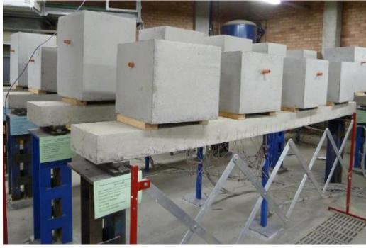
Fig. 2 Loading blocks arrangement and LVDT positioning for flexural test of SCC and FRSCC slabs
