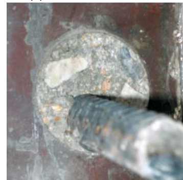
(c) Dowel shear with rebar
