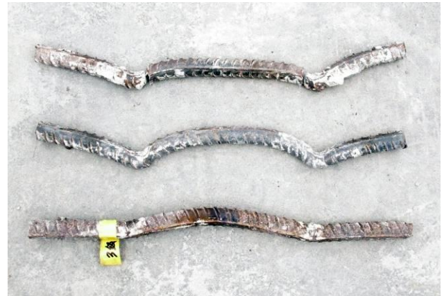
(b) Deformation of rebar
