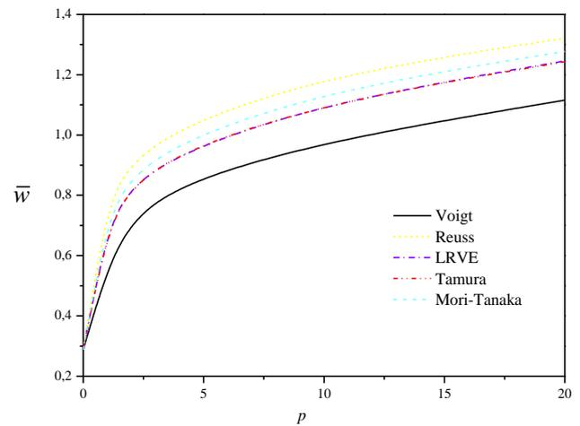
Fig. 4 The transverse displacement  $\bar{w}$  versus the power law index " $p$ " of FG square plates for different micromechanical models ( $a/h=10$ )
