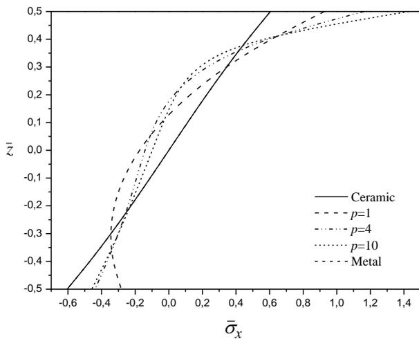
Fig. 6 The in-plane longitudinal stress  $\bar{\sigma}_x$  through the thickness of a FG rectangular plate ( $a/h=10$ ) -Voigt model-
