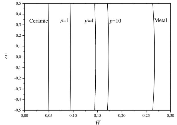
Fig. 3 The transverse displacement  $\bar{w}$  through the thickness of FG plates ( $a/h=10$ ,  $a=2b$ ). Voigt model
