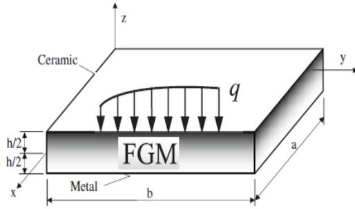
Fig. 1 Geometry of rectangular FG plate and coordinates
