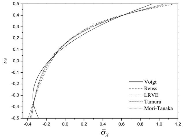
Fig. 7 The in-plane longitudinal stress  $\bar{\sigma}_x$  through the thickness of a FG rectangular plate for different micromechanical models ( $a/h=10, a=2b, p=1$ )
