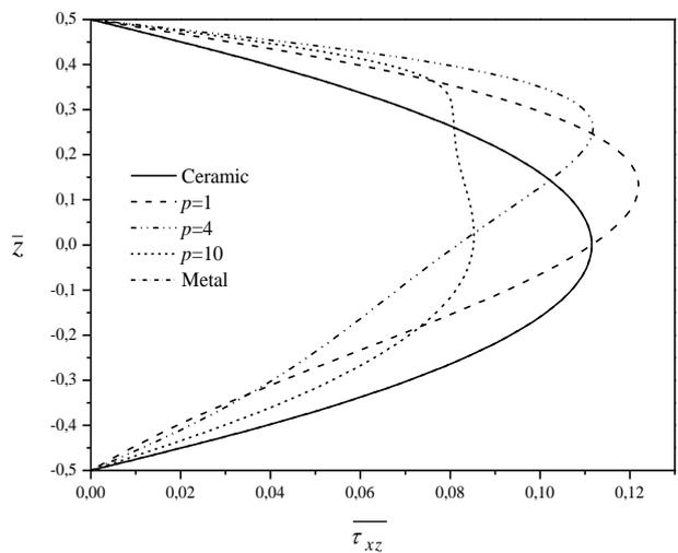
Fig. 8 The transverse shear stress  $\bar{\tau}_{xz}$  through the thickness of a FG rectangular plate ( $a/h=10, a=2b$ ) -Voigt model-
