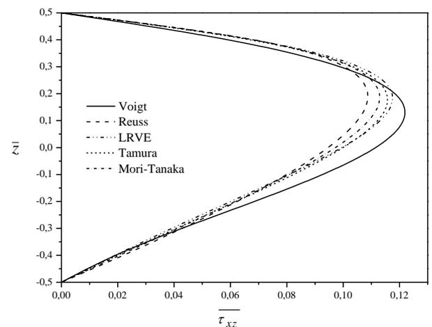
Fig. 9 The transverse shear stress  $\bar{\tau}_{xz}$  through the thickness of a FG rectangular plate for different micromechanical models ( $a/h=10, a=2b, p=1$ )
