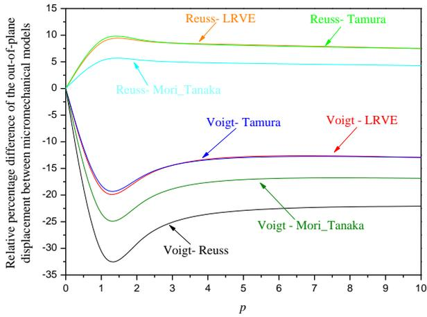
Fig. 5 Relative percentage difference between the micromechanical models of the transverse displacement  $\bar{w}$  of FG square plates ( $a/h=10$ )
