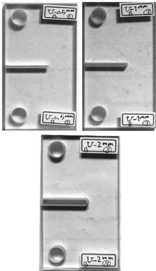
Fig. 3 U-notched GPPS samples with different notch tip radii of 0.5, 1 and 2 mm
