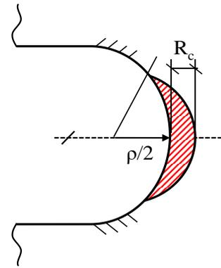
Fig. 5 Control volume for U-notch under mode I loading condition
