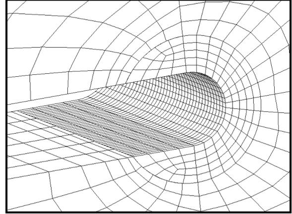
Fig. 6 Typical mesh pattern of the finite element model near the notch tip
