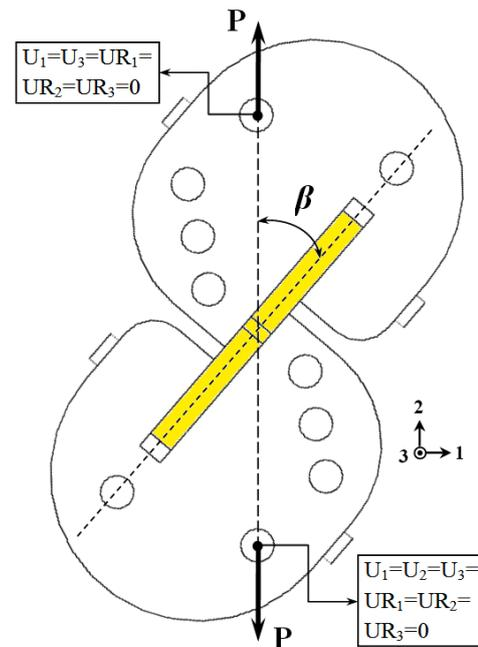
Fig. 1 Loading apparatus of mixed mode I/III fracture experiments
