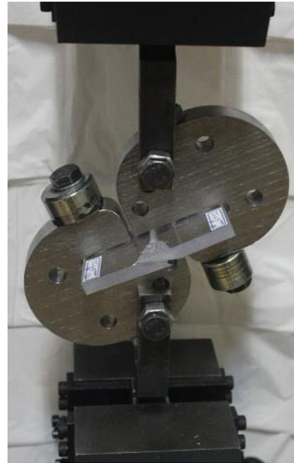
Fig. 4 The test configuration image showing the specimen fractured under the mixed mode loading case of  $\beta = 65^\circ$
