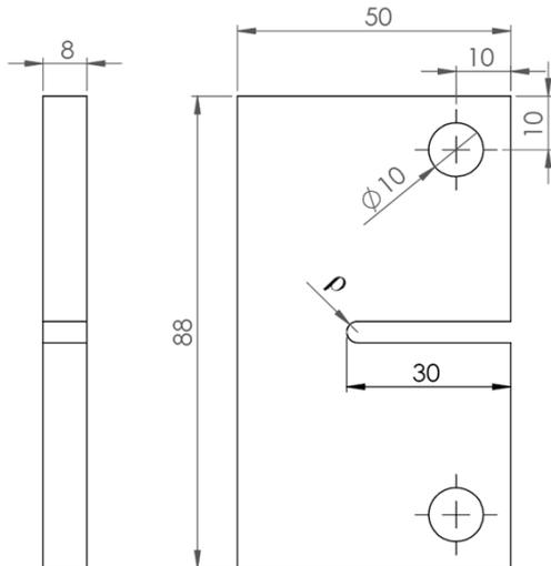
Fig. 2 U-notched specimen (dimensions in mm)
