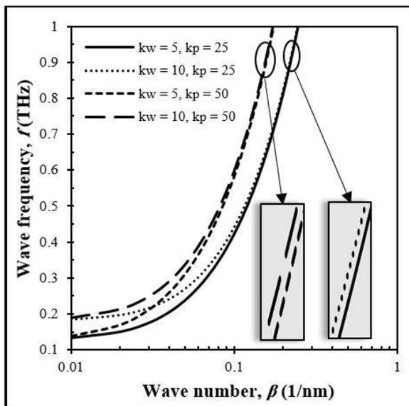
Fig. 5 Coupled effect of Winkler and Pasternak coefficients on wave frequency of DLGSs ( $\mu=\eta=0.1$  nm,  $C_d=0$ ,  $\Delta T=\Delta C=0$ )
