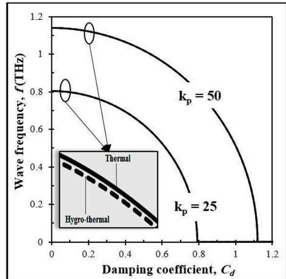
Fig. 9 Variation of wave frequency of a DLGS versus damping coefficient for various Pasternak coefficients and both thermal and hygro-thermal conditions ( $\mu=\eta=0.1$  nm,  $k_w=0$ ,  $\beta=0.2$ )
