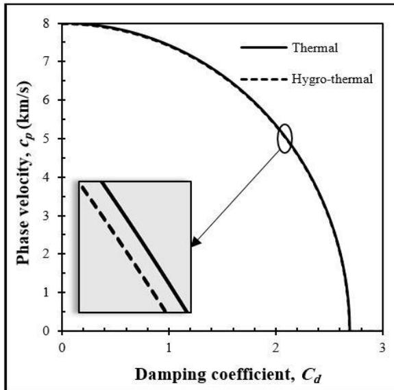
Fig. 7 Variation of phase velocity of a DLGS versus damping coefficient for both thermal and hygro-thermal conditions ( $\mu=\eta=0.1$  nm,  $k_w=k_p=0$ ,  $\beta=2$ )
