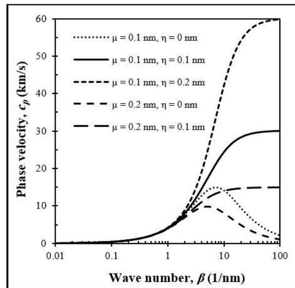
Fig. 3 Coupled effect of nonlocal and length scale parameters on phase velocity of DLGSs ( $k_w=k_p=0$ ,  $C_d=0$ ,  $\Delta T=\Delta C=0$ )
