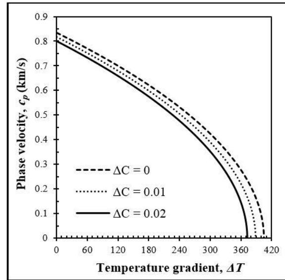
Fig. 6 Variation of phase velocity of a DLGS versus temperature gradient for different moisture concentrations ( $\mu=\eta=0.1$  nm,  $k_w=k_p=0$ ,  $C_d=0$ ,  $\beta=0.2$ )
