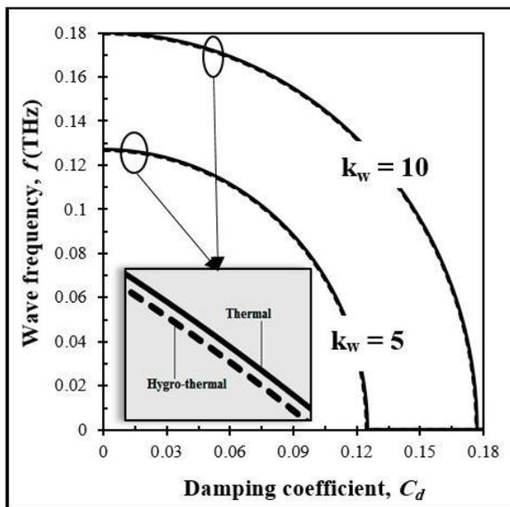
Fig. 8 Variation of wave frequency of a DLGS versus damping coefficient for various Winkler coefficients and both thermal and hygro-thermal conditions ( $\mu=\eta=0.1$  nm,  $k_p=0$ ,  $\beta=0.2$ )
