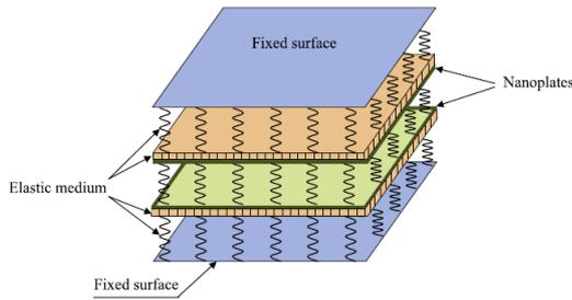
Fig. 1 Geometry of a double-layered graphene sheet rested on Winkler-Pasternak foundation
