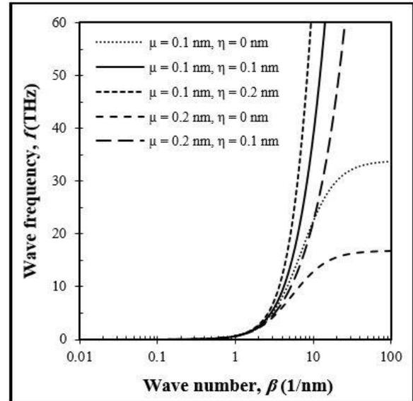
Fig. 2 Coupled effect of nonlocal and length scale parameters on wave frequency of DLGSs ( $k_w=k_p=0$ ,  $C_d=0$ ,  $\Delta T=\Delta C=0$ )
