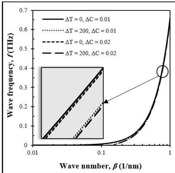
Fig. 4 Coupled effect of temperature gradient and moisture concentration on wave frequency of DLGSs ( $\mu=\eta=0.1$  nm,  $k_w=k_p=0$ ,  $C_d=0$ )
