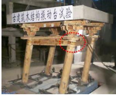
(a) Joints lateral movement
