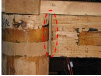
(b) The pulling out of tenon
