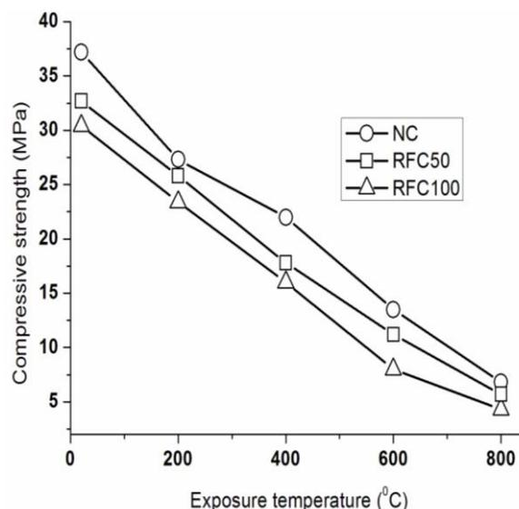
Fig. 4 Effect of elevated temperature on compressive strength of concretes
