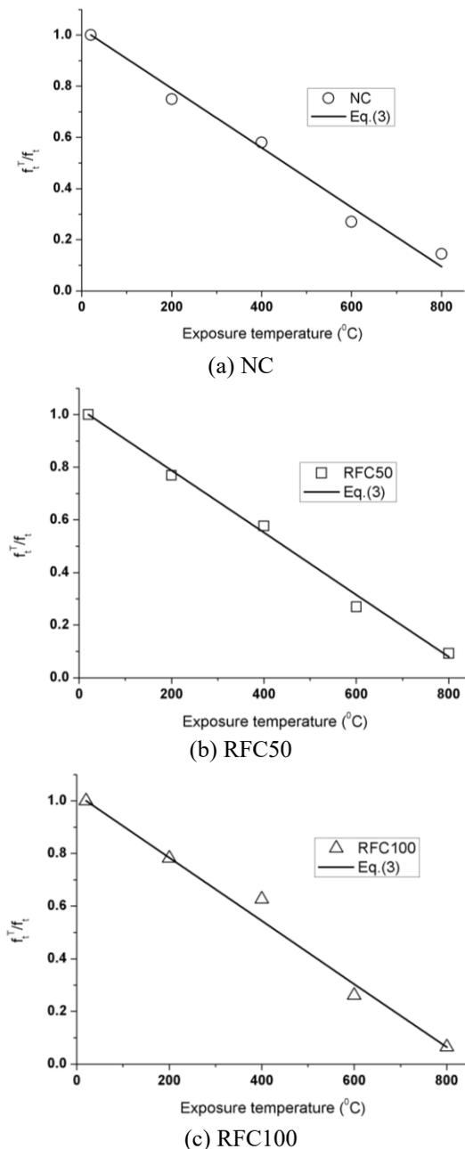
Fig. 9 Regress on the relationship between the residual split tensile strength and temperatures
