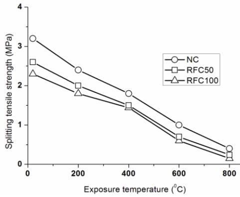
Fig. 8 Effect of elevated temperature on split tensile strength of concretes
