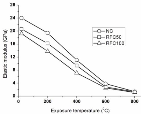
Fig. 6 Effect of elevated temperature on elastic modulus of concretes
