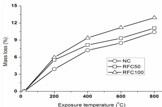
Fig. 3 Effect of elevated temperature on mass loss of concrete
