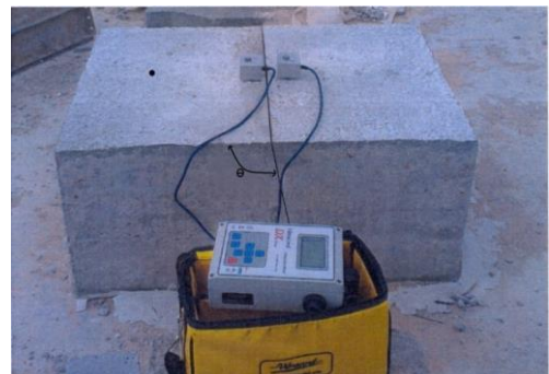
Fig. 2 A concrete block with a close angled discontinues
