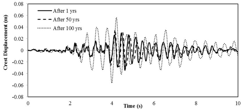
Fig. 8 Crest displacement of the Koyna dam at different age level from Washa *et al.* (1989)
