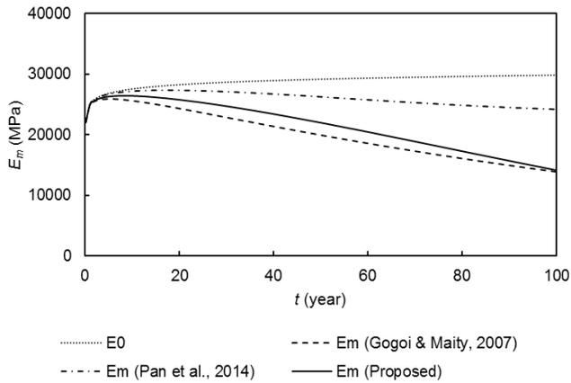
Fig. 4 Modulus of elasticity based on Dolen (2005) data
