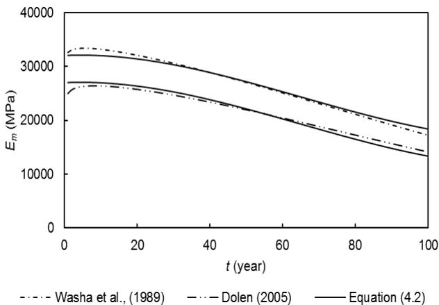
Fig. 5 Degradation concrete with time
