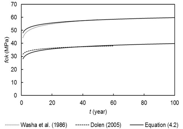
Fig. 2 Curve fitting of experimental data from Washa *et al.* (1989), Dolen (2005) for compressive strength
