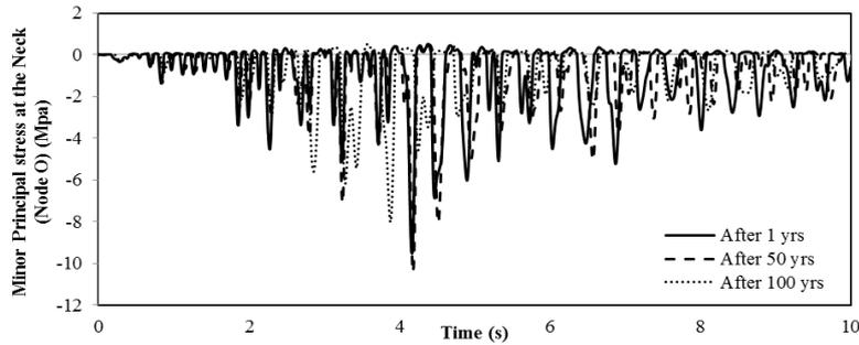
Fig. 15 Minor principal stress for three different age level from Dolen (2005)
