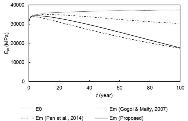
Fig. 3 Modulus of elasticity based on Washa *et al.* (1989) data
