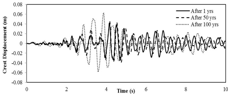
Fig. 13 Crest displacement of the Koyna dam at different age level from Dolen (2005)
