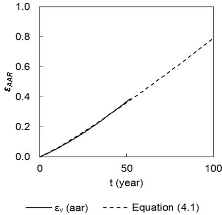
Fig. 1 Curve fitting of experimental data from Pan *et al.* (2013a) for expansion of AAR
