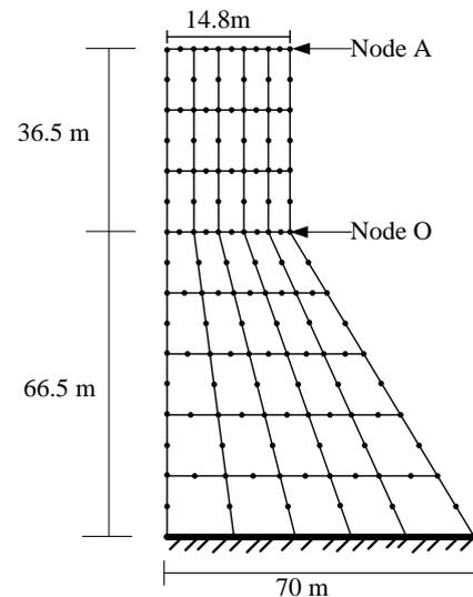
Fig. 7 Geometry and finite element discretization of Koyna dam
