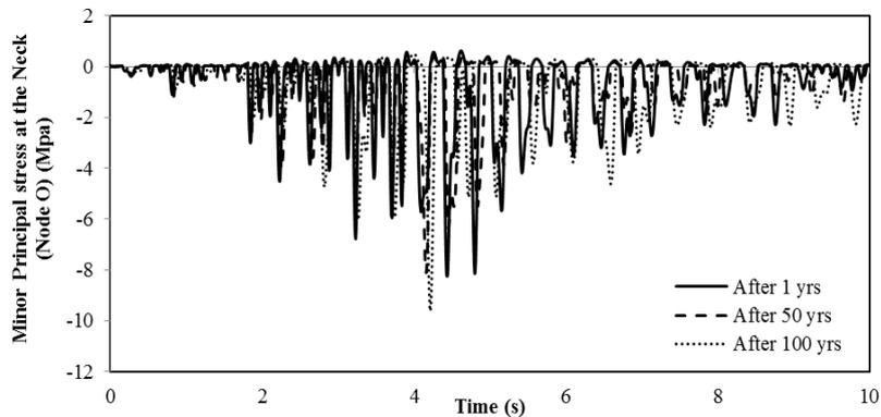
Fig. 10 Minor principal stress for different age level from Washa *et al.* (1989)
