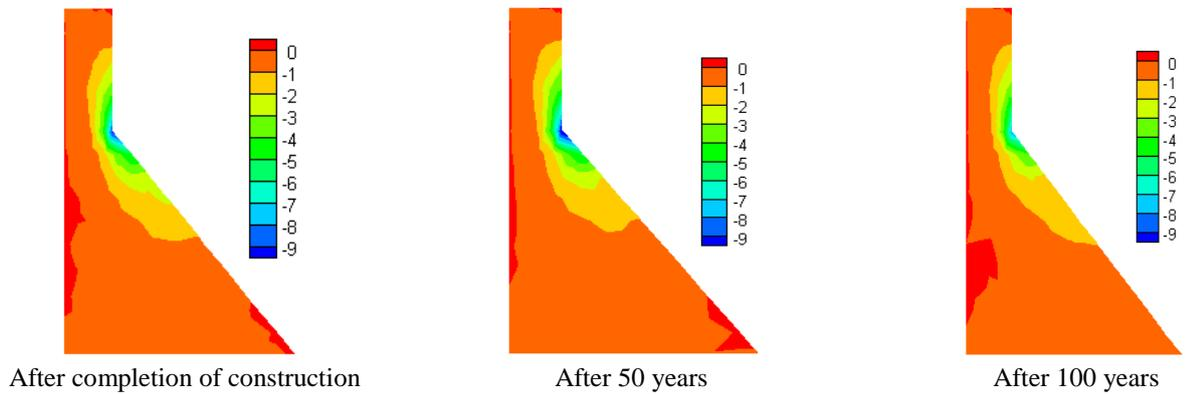
Fig. 17 Maximum minor principal stress contours for three different age level from Dolen (2005)
